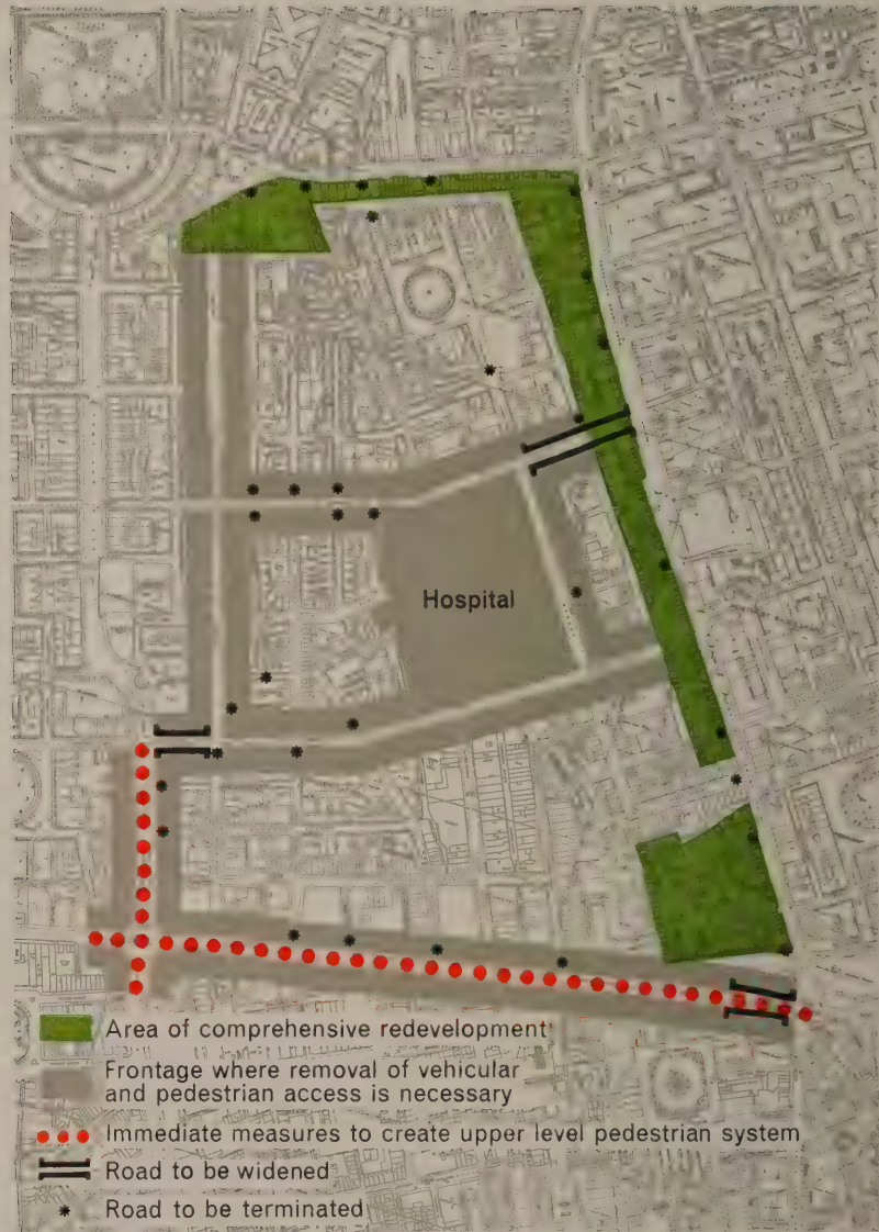
210 The scheme for minimum redevelopment. This figure shows the areas which would, in fact, require comprehensive redevelopment, and the frontages where redevelopment would need to be controlled in order, eventually, to separate pedestrians and vehicles.
